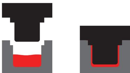
**Cast-forging** is a very special casting process. It is based on a low-turbulence filling of the mould. The molten metal gets carefully fed into an open, tempered mould and then cast under very high pressure.
