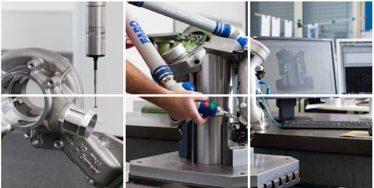
Measuring equipment – Gusstechnik Schopfheim: tactile measuring and
