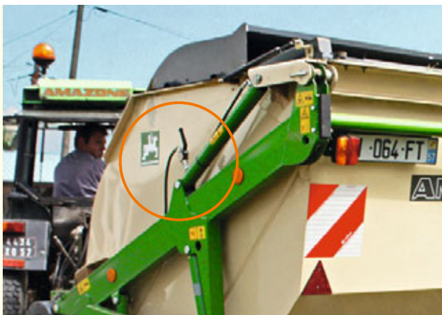
Hydraulic cylinder lock for Groundkeeper versions with high-lift emptying
