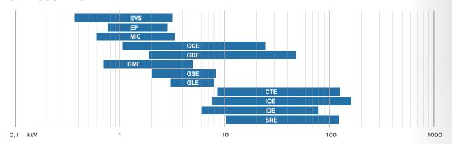
Nominal capacity: assessed in practical operating ambient, i.e. in wet conditions; R404A refrigerant; air inlet temperature 0 °C; evaporating temperature -8 °C; TD 8 K.
