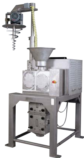
RC 250 with pneumatic lift device and two stage size reduction
