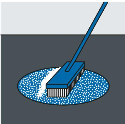
Clean the marking with a broom and use a sharp object to check that it is securely adhered. It can be walked and driven over after just a few minutes.
