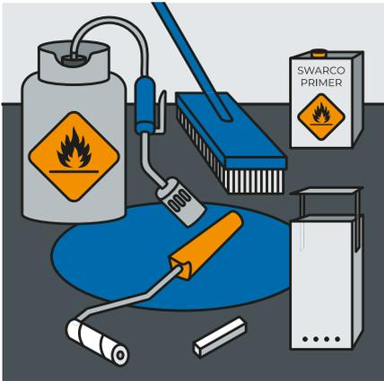
Equipment: Torch, broom, piece of chalk and drop-on material. Use a primer if necessary.
