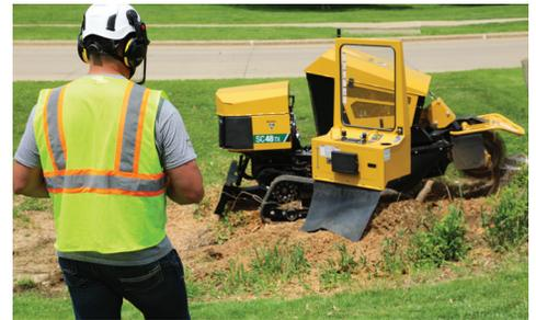
**OPTIONAL REMOTE CONTROL.** The optional full-function remote control allows you to operate the stump cutter without being at the operator's station, giving you jobsite flexibility.
