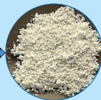
calcinated caolin with 1% silane
