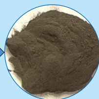
aluminum powder with 0,5% stearic acid
