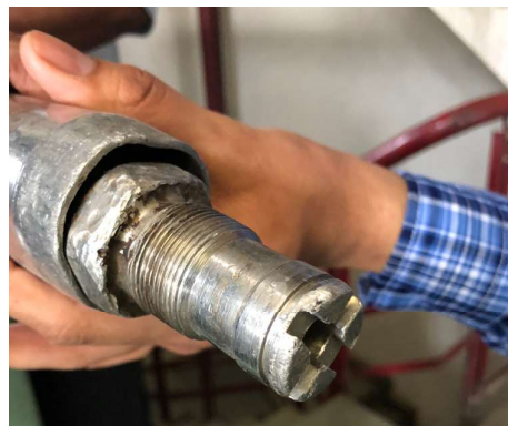
Damage to threads on SDX® III Nozzle.
