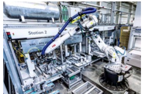
Leak testing of the fully assembled components
