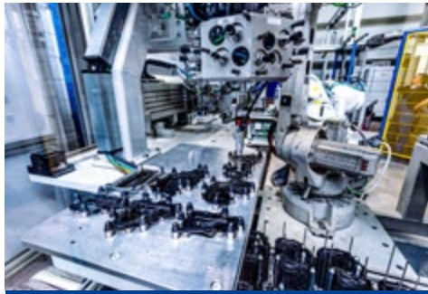
Automated removal of the sheet metal covers
