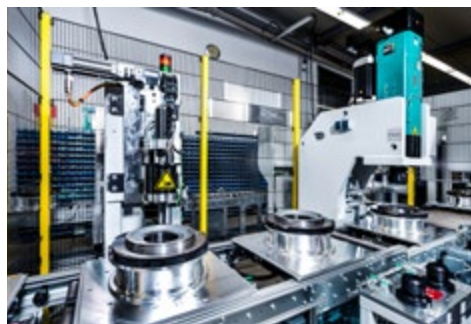
entering the measuring station including DMC-reader and DIATEST measuring system
