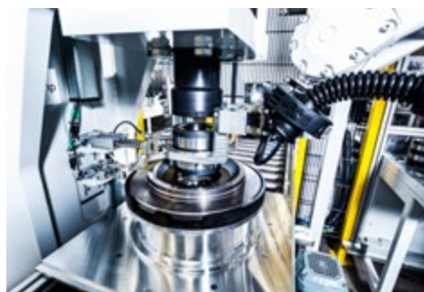
temperature difference <2^{\circ}\text{C} : pressing in with forces up to 150 kN
