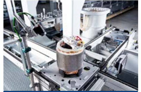
position control of the stator via camera
