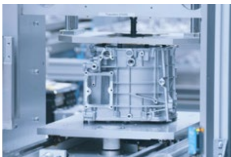
HA-P: Inductive heating and joining of the bearing bushing from below
