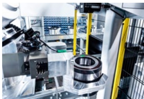
withdrawal of the bearing via robot and automatic DMC-reading of each part
