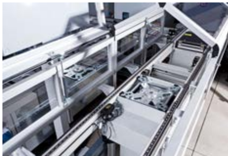
cooling tunnel with covers including access facilities
