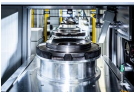
measured curve is OK: transport to the laser cabin for DMC-reading and laser marking with the collected data
