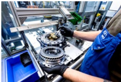
HA: Manual pre-assembly of the heat sinks, followed by automatic assembly
