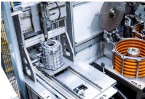
HA: Screw connection of the heat sink with parameter monitoring
