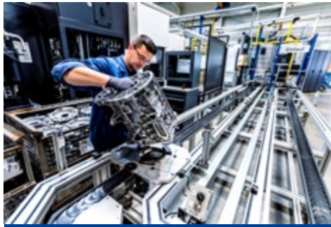
Possibility of direct component infeed via circulation belt
