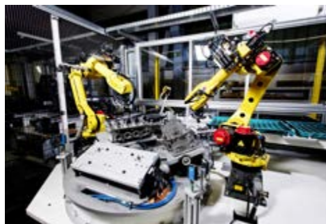
HVA element and roller cam followers assembly
