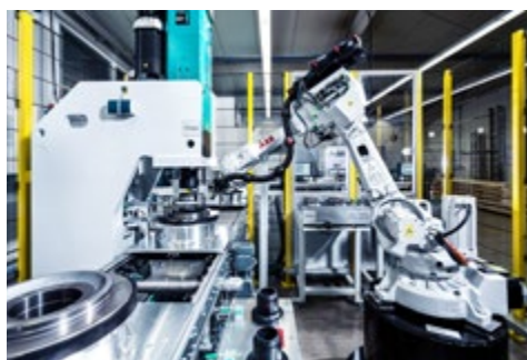
positioning of the bearing for temperature measuring
