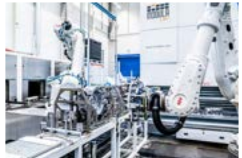
Loading of impregnation racks
