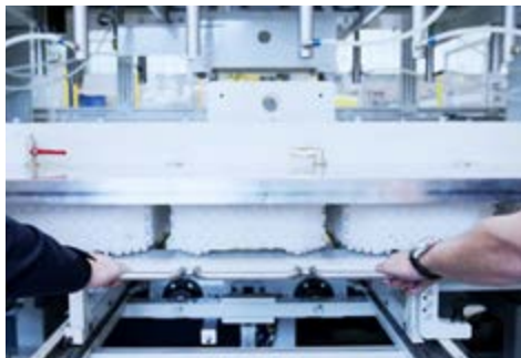
integrated maintenance mode for changing the upper sealing plate
