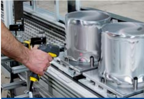
transfer of the component from premachine, if necessary merge of rework parts via DMC hand scanner
