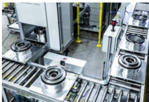
in case the measured force/stroke curve is NOK: transport to the NOK stopper, no laser marking takes place
