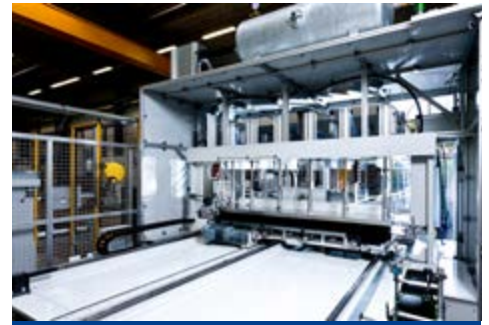
air leak test with small test pressures
