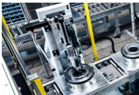
testing diameters regarding different drill depths
