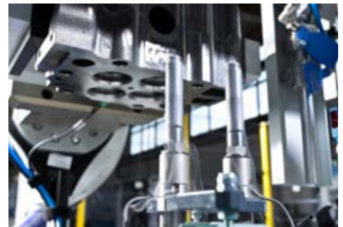
Pressing in of nitrogen-cooled valve guides
