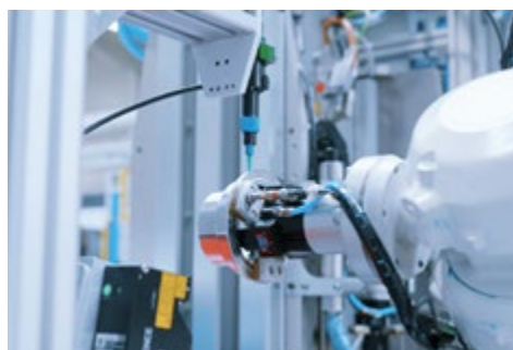
VA: Automatic sealant application incl. control by means of 3D scanner
