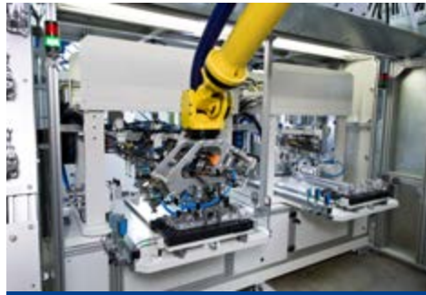
Cylinder head cover leak testing
