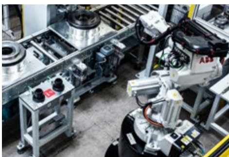
temperature difference >2^{\circ}\text{C} between housing and bearing: positioning on the NOK-storage
