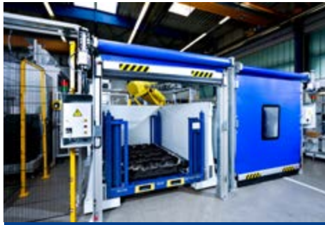
part loading with special rack
