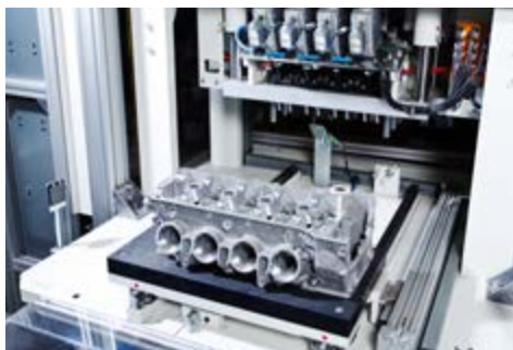
Hammering in valves and leak testing
