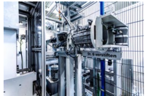
Clamping of the component as well as automatic pinning
