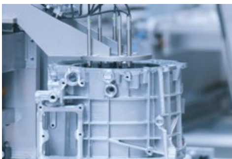
HA-P: Dimensional control of the joining position, followed by transfer for further processing
