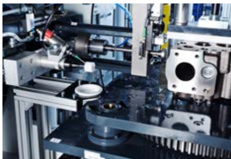
Loctite wetting and pressing in of threaded bushings and closure caps
