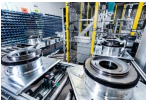
inward transfer via separating stops
