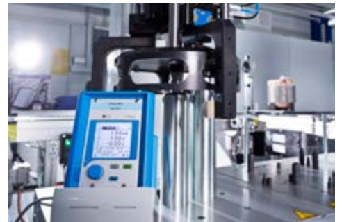
automated counter measuring device for the joining axis
