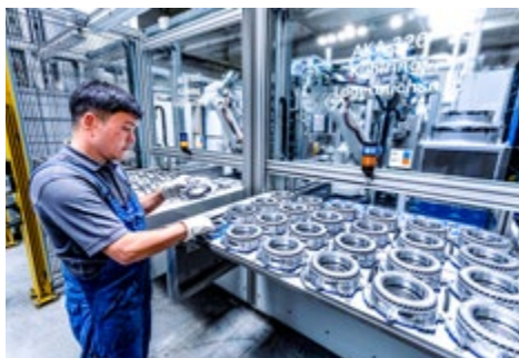
HA: Manual loading of the feeder drawer for heat sinks and bearing bushings
