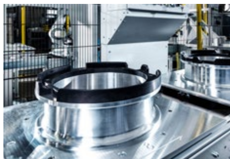
quality of the DMC is OK: transport of the assembled component to the unloading stopper
