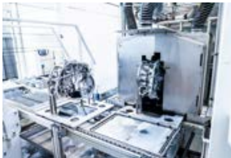
Further transport of the machined components into the washing cell
