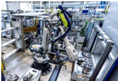
Deposit in rack system for curing of sealant and transfer to cell 6
