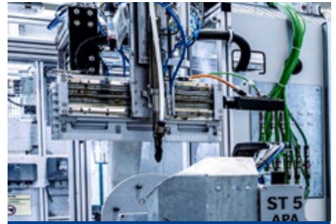
Positioning and screwing the sheet metal covers
