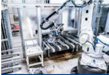
Discharge of N.O.K. components
