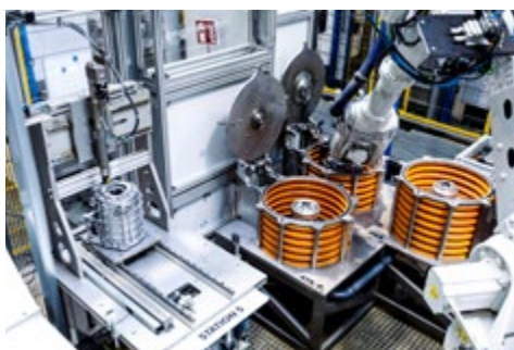
Removing a component (front axle VA) from pre-cleaning
