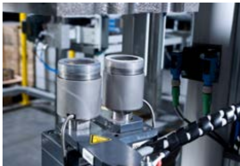
Pressing in of nitrogen-cooled valve seat rings
