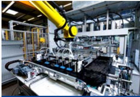
application of a handling-robot with vacuum gripper system
