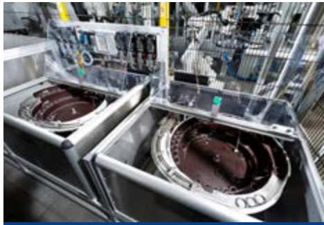
Automatic supply of valve seat rings
