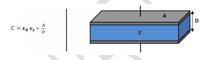
Capacitance is proportional to the area of overlap but inversely proportional to the separation between the conducting sheets. The bigger the area of overlap is and the closer the sheets are to each other, the greater is the capacitance.
