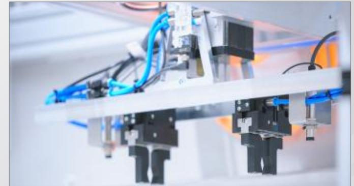
Greifer an Mehrachs handling | Gripper on multi-axis handling
