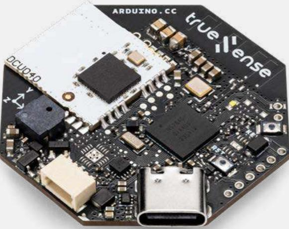
Designed to work in combination with the Portenta UWB Shield, Arduino Stella elevates your IoT projects by leveraging UWB technology for unparalleled accuracy and seamless integration. Featuring the advanced nRF52840 microcontroller and Truesense DCU040 module, Stella is the ultimate tool for real-time tracking, automated safety systems, and intuitive human-machine interactions.
