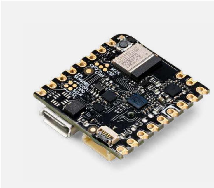
Implement **always-on speech recognition on the edge** with Nicla Voice. The board integrates a **Neural Decision Processor™** from Syntiant, allowing to run multiple AI algorithms.
