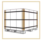
Vertical use enhances pallet durability and prevents products from being crushed or scattered.
