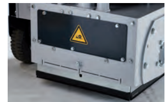
Tool-near marking of the working width of 400mm - Easy orientation
