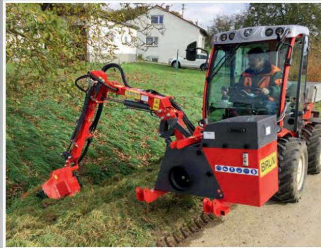
Bruni Dual boom with mulching head
