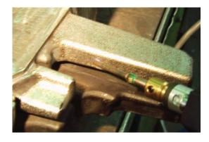
Runners, Overflows, and Vents - The vents on a die stay much cleaner when they have received a carbide coating. Minor cracks in the die can be Rocklinized as long as they haven't gotten too wide.
