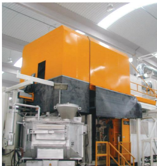
■ Hood into two parts complete with ENERPRESS filtration system, fan and individual expulsion into the atmosphere on ITALPRESSE IP1650 die-casting machine - Spain
