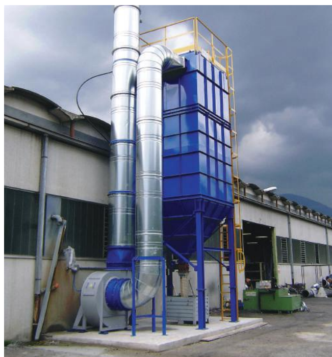
■ Fume suction and filtration system (flow rate 20,000 m 3 /h) for aluminum smelting furnaces - Italy
