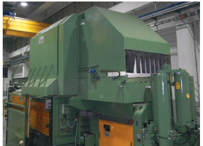
■ Hood on Hydra press connected to ENERPRESS centralized suction and filtration system - Italy
