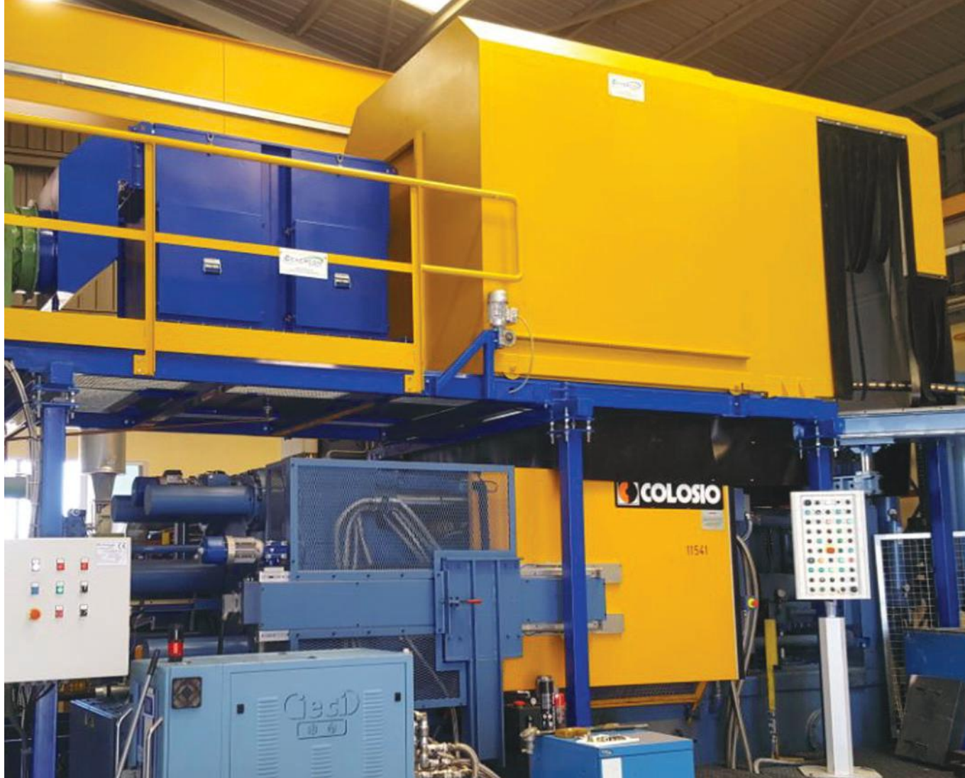
■ Hood into two parts complete with individual ENERPRESS filtration system, fan and individual chimney for the expulsion in the atmosphere of purified air on COLOSIO PFO560 die-casting machine - Spain
