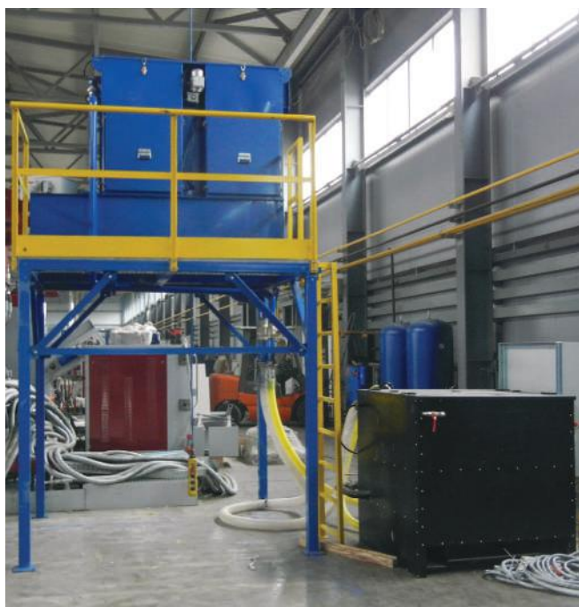
ENERPRESS filter on an independent structure with mobile washing tank beside it, dedicated to a single die-casting machine and connected to a centralized suction unit. Ukraine
