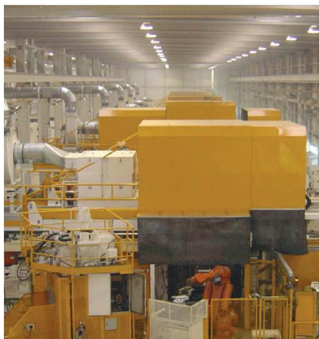
■ Die-casting machines with hoods in two parts complete with ENERPRESS filters, fans and individual chimneys for the expulsion of air purified in the atmosphere - Spain
