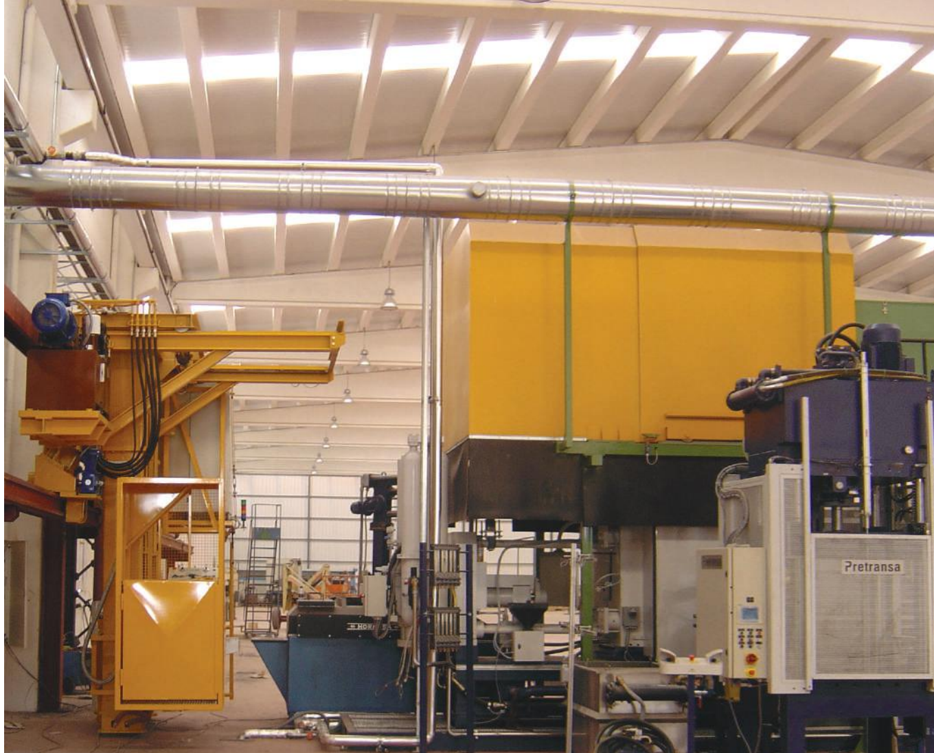
■ Automatic ladle wagon for the pouring of aluminum into holding furnaces at the service of die-casting machines - Spain
