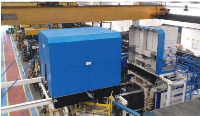
■ Hood into two parts on IDRA OL900S die-casting machine complete with individual ENERPRESS suction and filtration system, mobile hood on the injection side - Spain
