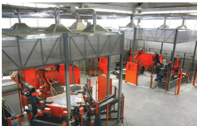
■ Extraction hoods on gravity casting cells connected to a centralized suction and filtration system - Italy
