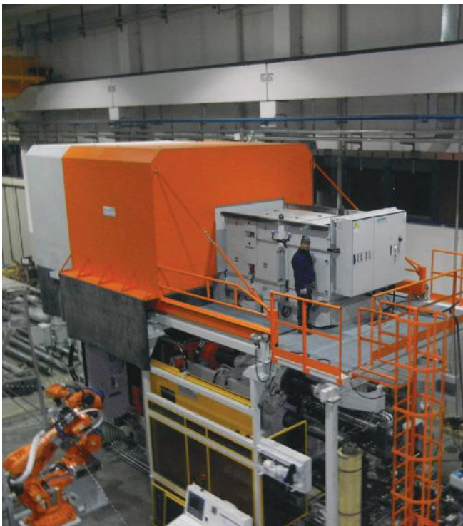
■ Hood into two parts complete with individual ENERPRESS suction and filtration system for recirculation of purified air in a die-casting machine - Russia
