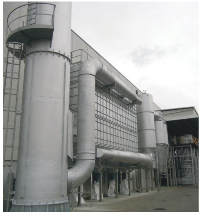
■ Fume suction and filtration system from aluminum melting furnaces with chemical treatment of the fumes in the reactor and reagent storage and dosing system - Italy
