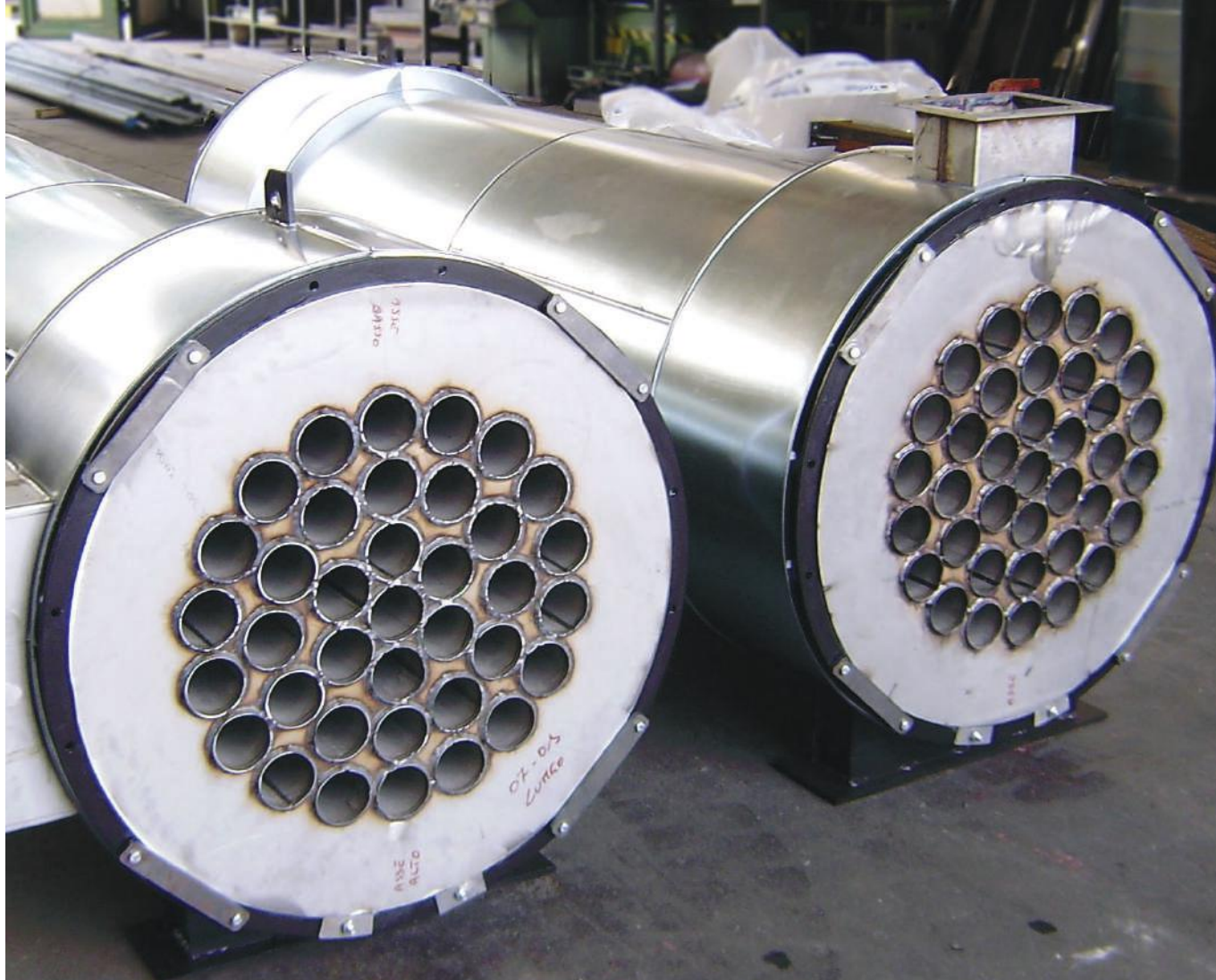
■ Tube bundle heat exchanger (fumes/air) for preheating combustion air before placing in the furnace - Italy
