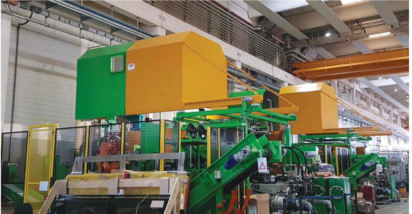
■ Hoods on presses connected to a centralized suction and filtration system - Uzbekistan
